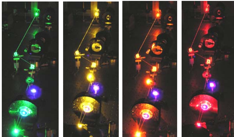
Femtosecond optical parametric oscillator spanning across the full visible spectrum.
